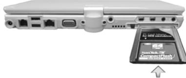
To eject a PC card, push on the tip of the rod with your fingertip, and then push the rod to eject the card.
