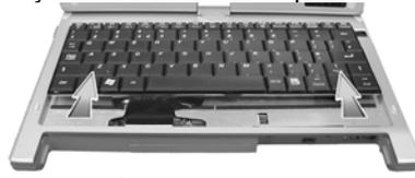
**4** Gently release the lock mechanism of flat cable connector with your fingertips and then take the keyboard out.
