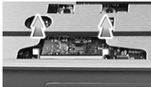
**3** Insert the flat cable into flat cable connector, make sure it is fully inserted, and then push the lock mechanism with your fingertips to lock it.
