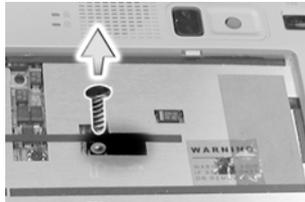
**2** Hold the base of computer with your hands, gently tilt the computer's back side upwards slightly, clasp the hard cover with your right hand's fingertips, and then pull the hard disk set out with your right hand gently.
