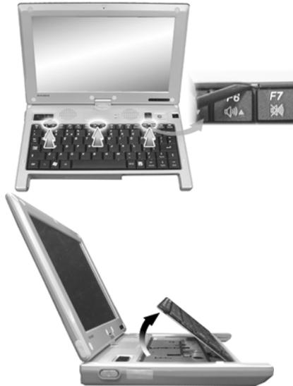
**3** Gently move the keyboard forwards until the flat cable of keyboard is fully stretched, and then put the keyboard down on the top cover.
