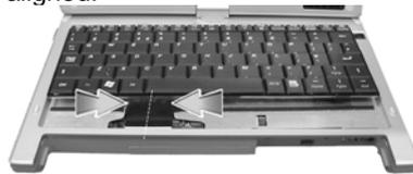
**2** Check and adjust the lock mechanism of flat cable connector. Make sure it is in fully released condition.
