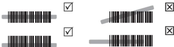
To scan a barcode, make sure the aiming beam crosses every bar and space of the barcode. For fixed mounted scanning, Continuous Mode(see **READING MODE**) is recommended.
