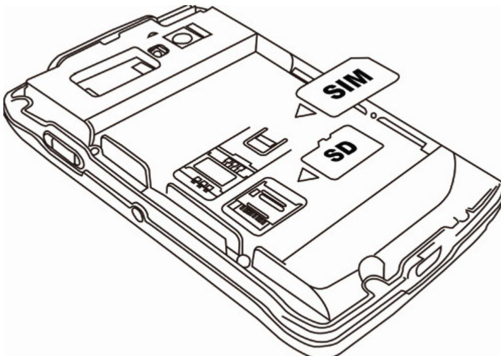
5. Push the metal cover backward and lift the metal cover. Then put the SD card into the socket, close the metal cover and push forward till click sound.
