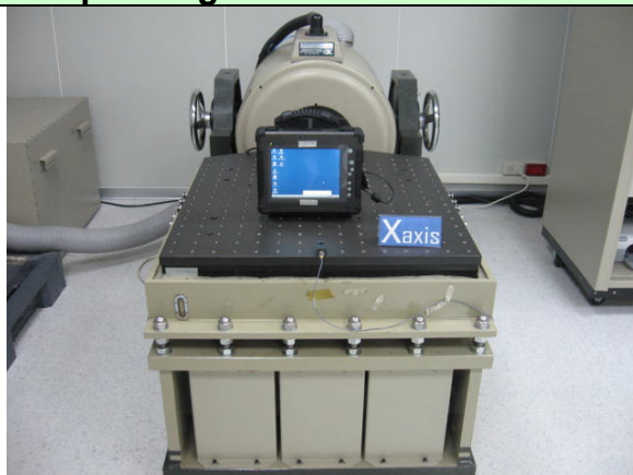
Operating Vibration Test—X axis
