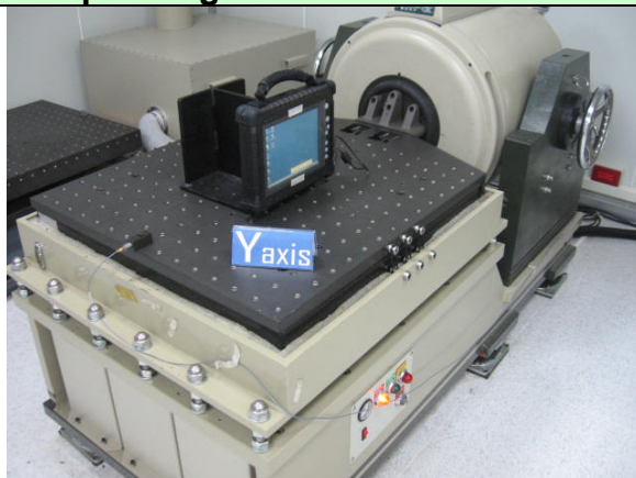
Operating Vibration Test—Y axis
