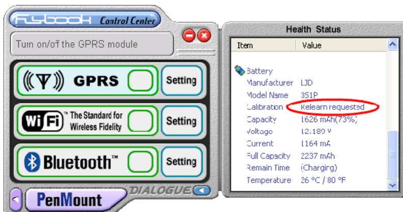
3. If the [Calibration] column displays [Relearn requested] message , the battery need to calibration.
