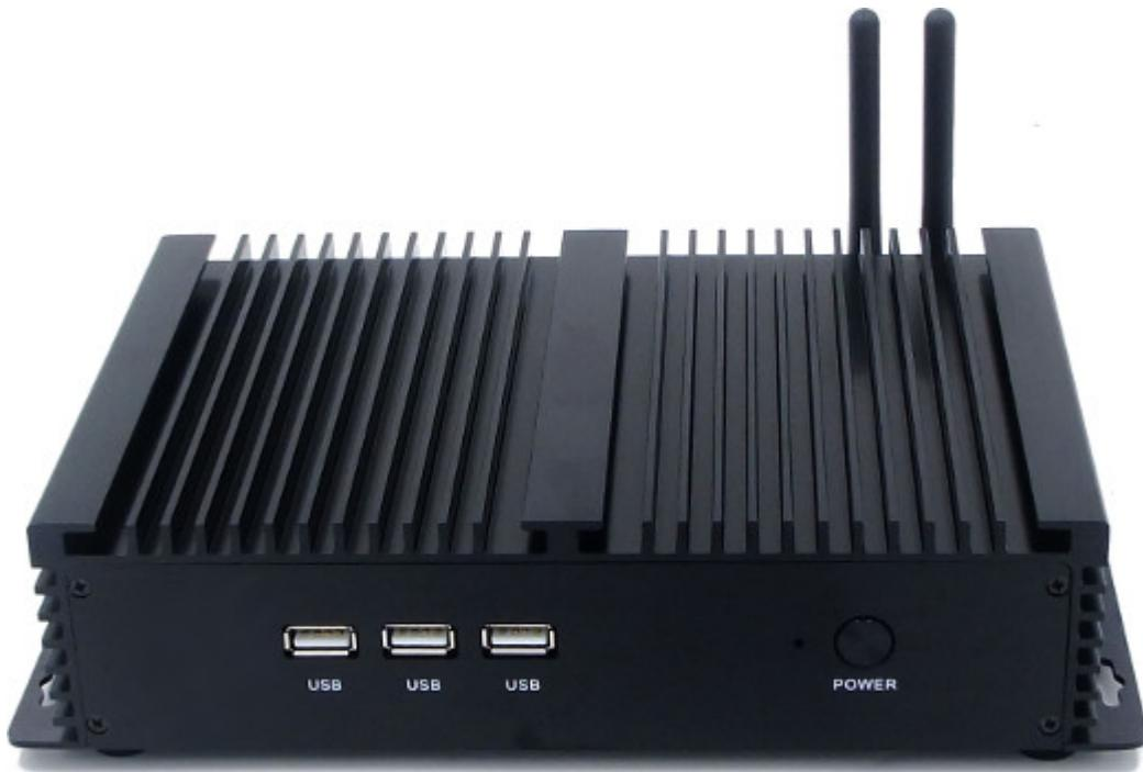
Integrated card - **Intel RTL8186/8111/8112 Gigabit NIC** and the **Wi-Fi** module allow connection to the network. The computer is equipped with: one **LAN** port, one **VGA** port, one **HDMI** port, four **USB 3.0** ports, three **USB 2.0** ports, two **COM(RS232)** ports, one **Mic** and one **Speaker** port and a built-in connector on the motherboard: **SATA** port and **mSATA** port.
