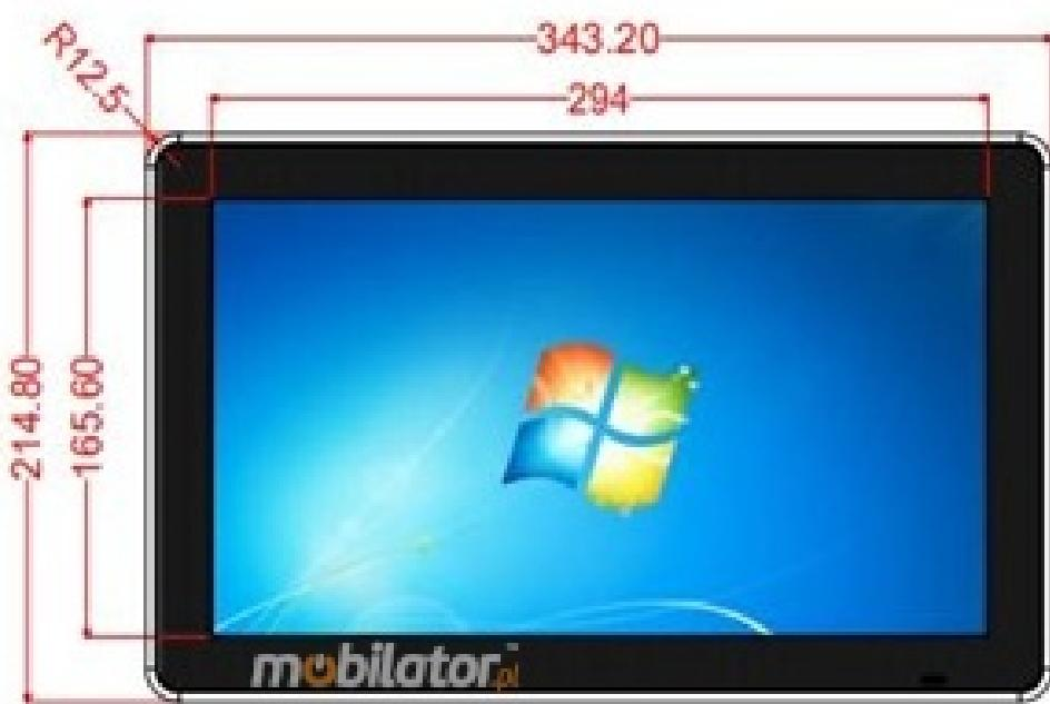
The BiBox 133-I58 is a durable panel computer designed for efficient outdoor use. Its screen boasts a brightness level of 250 nits, which is crucial for excellent readability in shaded areas or in moderate sunlight. This
