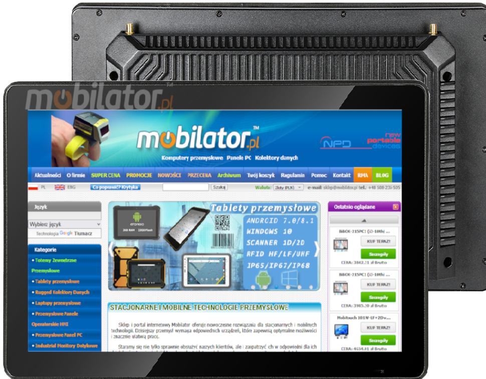
The BiBox 17-I510 device has been designed to operate in demanding environmental conditions. It is characterized by the ability to operate in a wide temperature range from -10°C to 60°C and high resistance to relative humidity up to 95%, in the absence of condensation. Additionally, the equipment can be safely stored at extreme temperatures, from -20°C to 70°C, ensuring reliability in various operating conditions.
