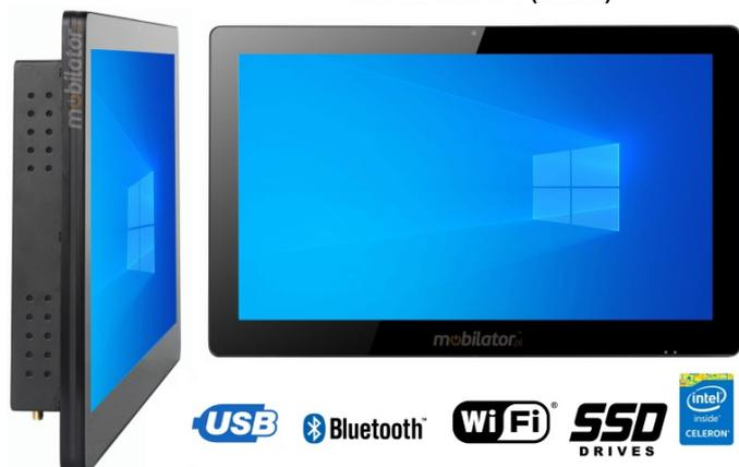
BiBOX-185PC1 (J1900) v.5 - Powerful panel computer with touch screen, IP65 resistance, WLAN network and extended SSD (512 GB)
