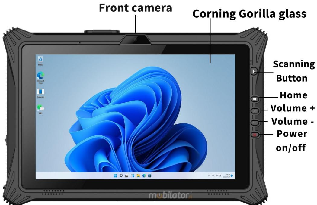
The dustproof Emdoor I10A is equipped with a touch panel with Corning Gorilla glass, a set of physical buttons (volume, Home, scan, power) and a modular expansion slot (RJ45 / RS232 / USB / 2D). The back of this functional tablet is protected by a reinforced casing, a battery lock and optional modules: NFC and a fingerprint reader.
