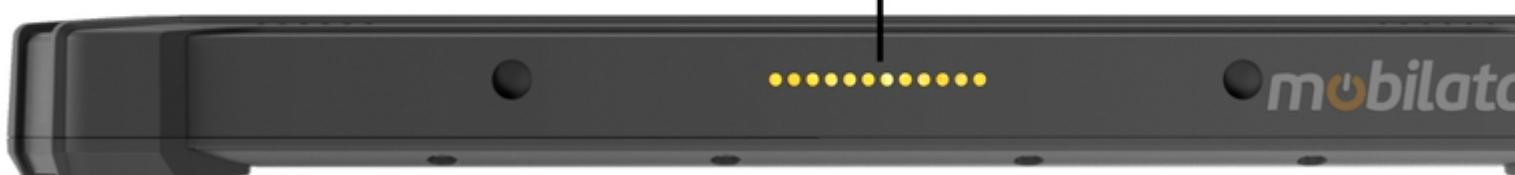
The POGOPIN connector allows you to quickly connect a military tablet to the docking station.
