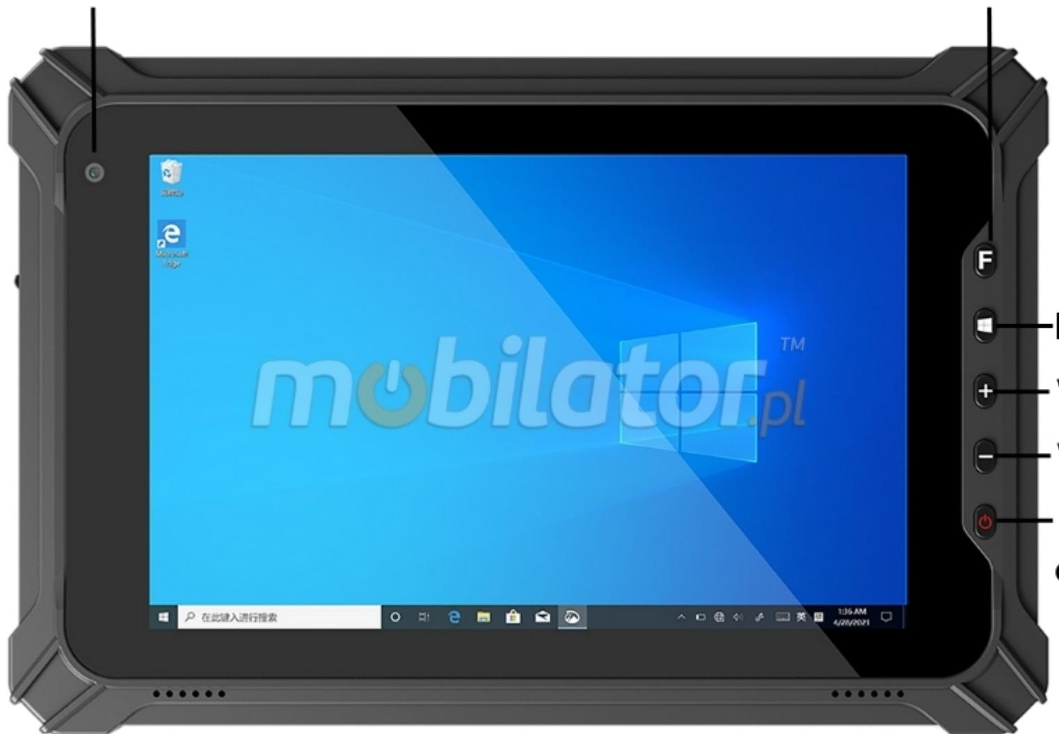
The extremely durable Emdoor I87J features a set of physical buttons (volume, home, and one programmable button).
