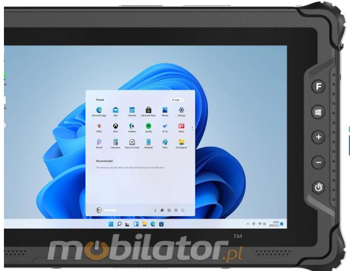
Emdoor I88N v.10 - Multitasking industrial tablet with NFC, GPS, 2D barcode scanner - with Windows 11 PRO license - compact and durable with IP65 rating
