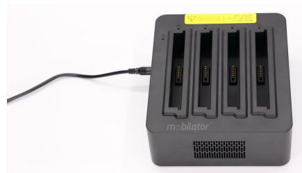
The docking station allows you to quickly and safely charge four batteries at once.
