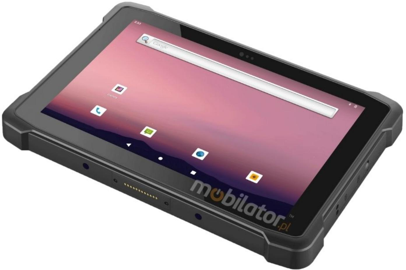
The IP65 standard, which this rugged tablet meets for demanding applications, defines the level of protection provided by the enclosure against access to hazardous internal components, ingress of solid objects, and exposure to splashes or water directed from any direction. Compliance with this standard ensures the Emdoor T11X military tablet remains highly resistant to operation in both industrial and outdoor environments, regardless of weather conditions.
