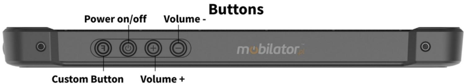
The exceptionally robust Emdoor T11X is equipped with a set of physical buttons including volume control, power switch and an additional programmable key that increases the functionality of the device and facilitates operation in demanding working conditions.
