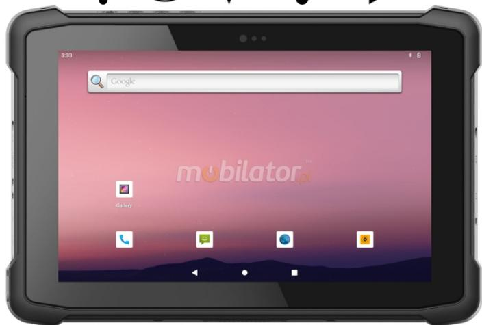
EMDOOR T11X v.2 - Rugged IP65 tablet with Android 12, 10-inch screen, 8GB RAM, LTE, GPS, Bluetooth, and 2D barcode scanner - perfect for mobile sales and inventory systems
