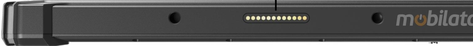
The POGOPIN connector allows you to quickly connect a military tablet to the docking station.
