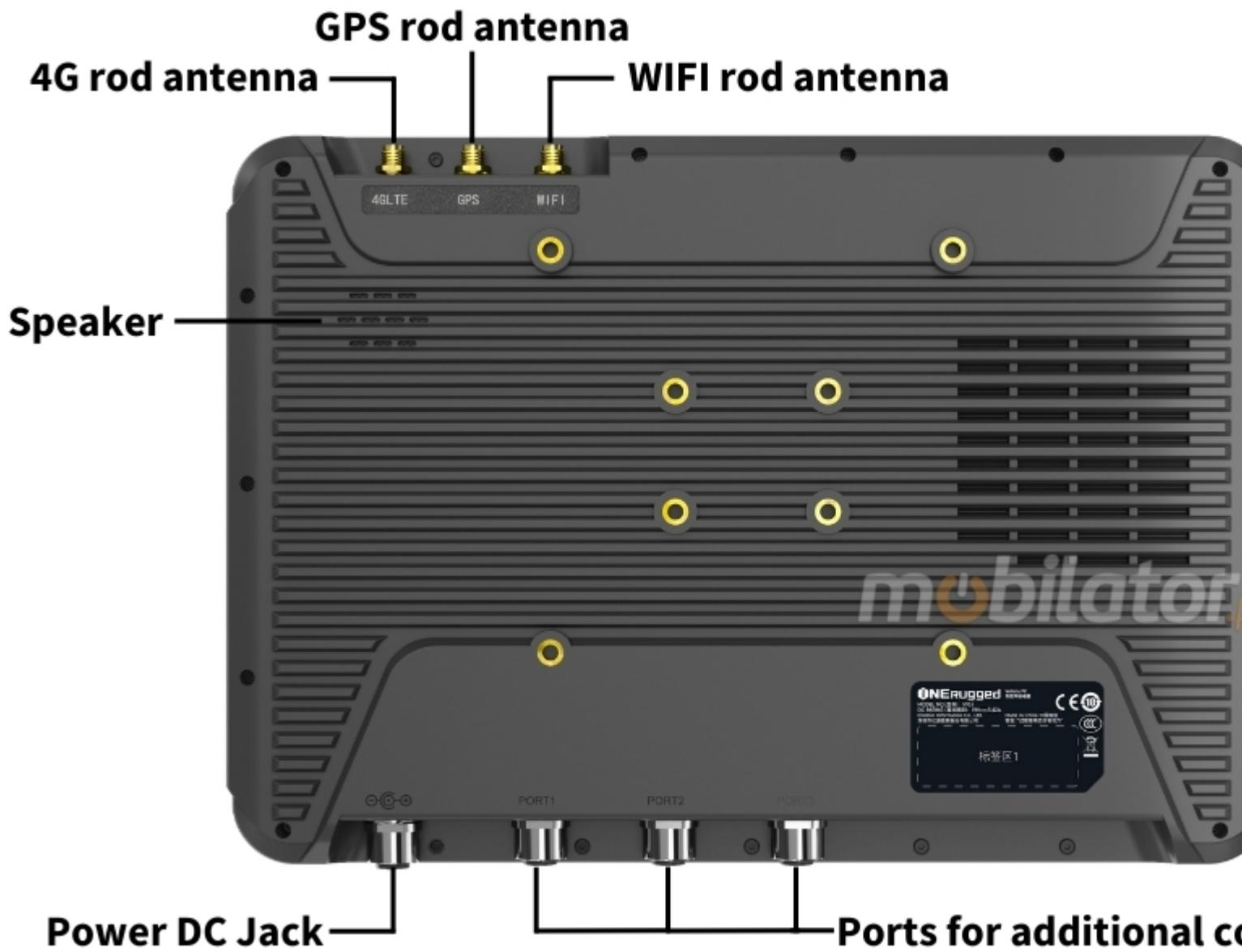
The splash-proof Emdoor V10J tablet offers built-in GPS, Wi-Fi, and 4G antennas\* (only works with 4G). Additionally, this ergonomic tablet features a DC power jack and ports for additional connectors (RS232, USB, RS485, and RJ45), which are available for purchase as accessories.
