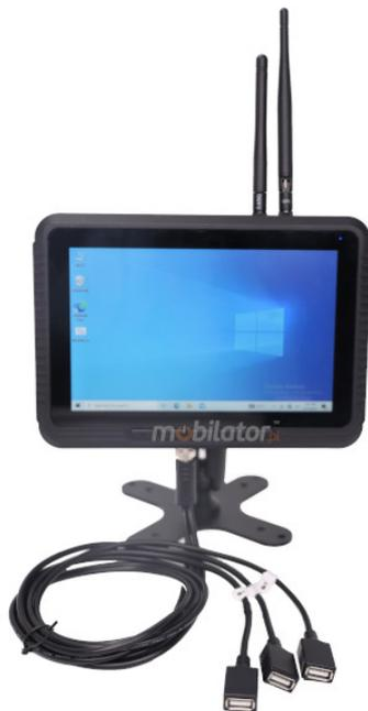
The cable required to obtain USB 2.0 and CAN connectors, enabling convenient and stable connection of devices.
