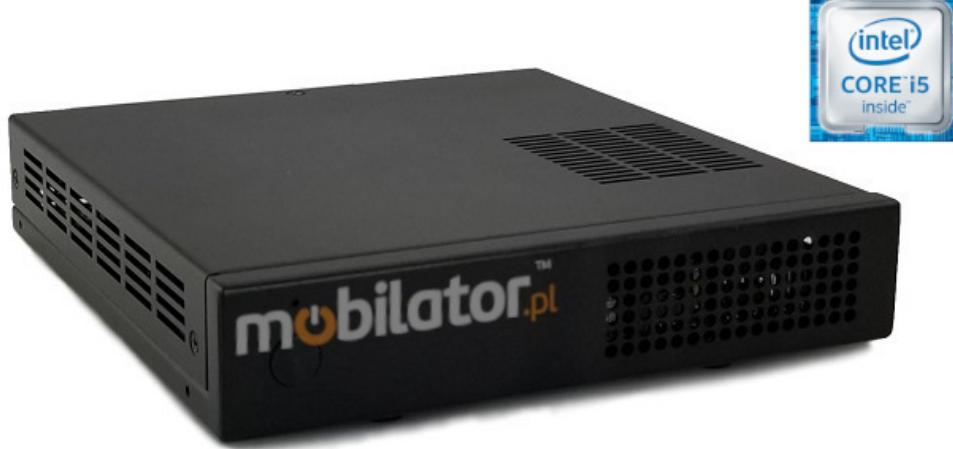
The industrial mini-computer Polywell HM170L4 i5 BARBONE uses an efficient and energy-saving Intel Core i5 processor. Inside it there are four cooperating cores enabling more efficient processing of many tasks at the same time. The shared cache memory in which the multilevel hierarchy is used is dynamically allocated to each processor core depending on the load. This reduces the average access time to the main memory.
