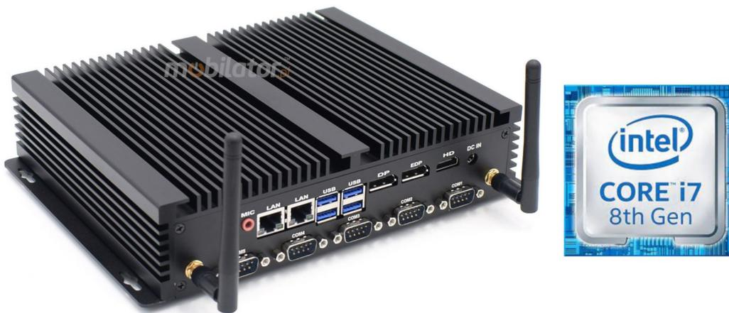
The industrial mini-computer HyBOX H4 uses an efficient and energy-saving Intel Core i7-8550u processor. Inside it there are four cooperating cores enabling more efficient processing of many tasks at the same time. The shared cache memory in which the multilevel hierarchy is used is dynamically allocated to each processor core depending on the load. This reduces the average access time to the main memory.
