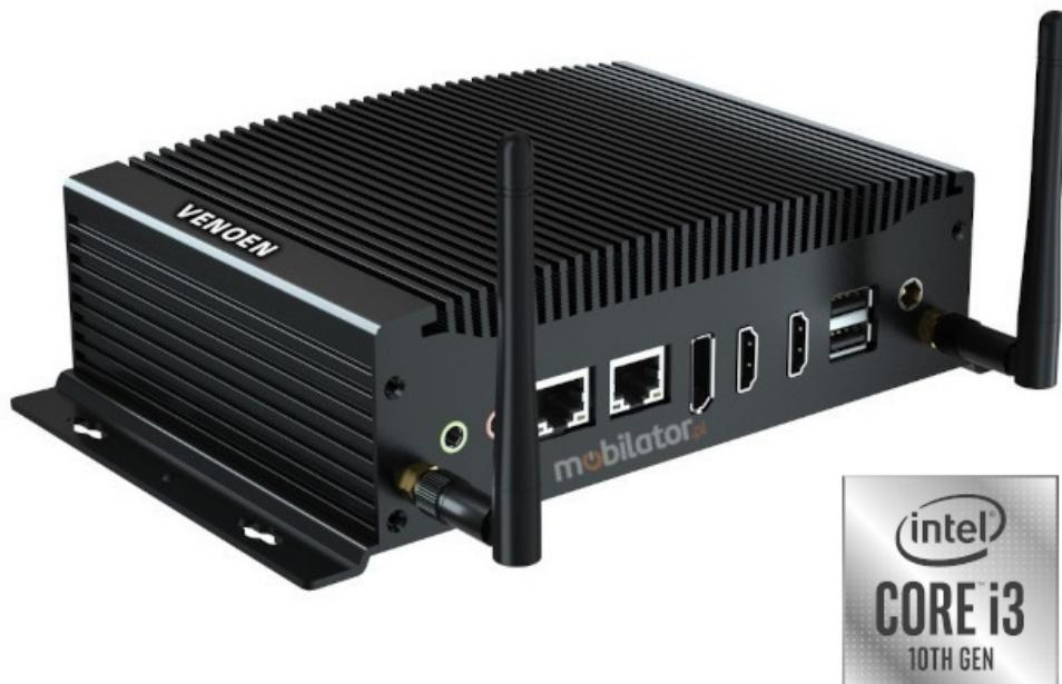
The industrial mini-computer HyBOX H6 - i3 uses an efficient and energy-saving Intel Core i3-10110U processor. Inside it there are two cooperating cores enabling more efficient processing of many tasks at the same time. The shared cache memory in which the multilevel hierarchy is used is dynamically allocated to each processor core depending on the load. This reduces the average access time to the main memory.
