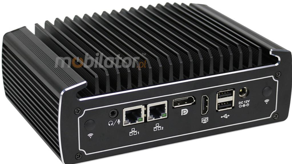
The industrial mini-computer IBOX 2203N uses an efficient and energy-saving Intel Core i7 10810U
