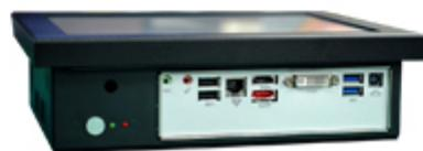
Industrial PanelPC D-SYS 10.4 has a water-resistant front panel and scratch resistant LCD screen. With 1024x768 resolution and high brightness of 350 cd/m<sup>2</sup>, screen of "4 wire resistive" type with high sensitivity to touch, offers the user a clear picture and ease of use.
