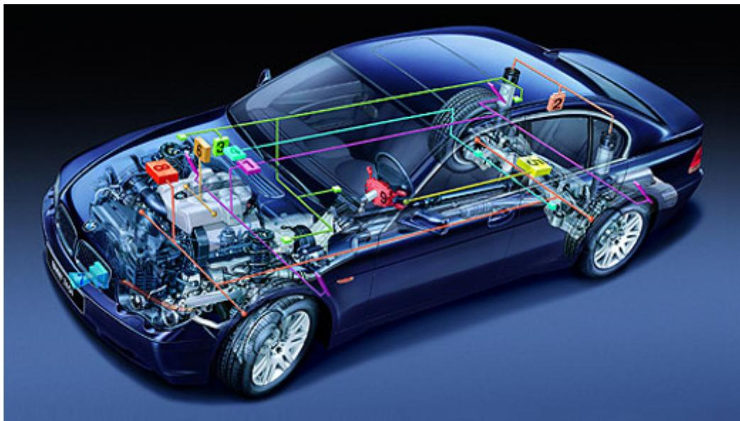
CAN is an asynchronous serial bus for data exchange. It has been designed for the automotive industry to increase the reliability of systems such as ABS and engine control. This is commonly used in a variety of fields, primarily in the automotive
