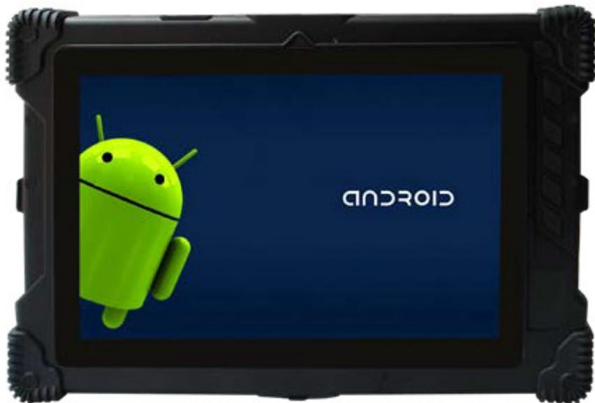
The display of the image corresponds to the 10.1-inch full touch screen (1280 x 800 XGA) LED-backlit display with Sunlight Readable Technology (350nit), Which uses reflected light beam as a light sensor - the bigger the better backlight illumination sensor. The Resulting display bright and is **easy** to read even in direct sunlight encounters.
