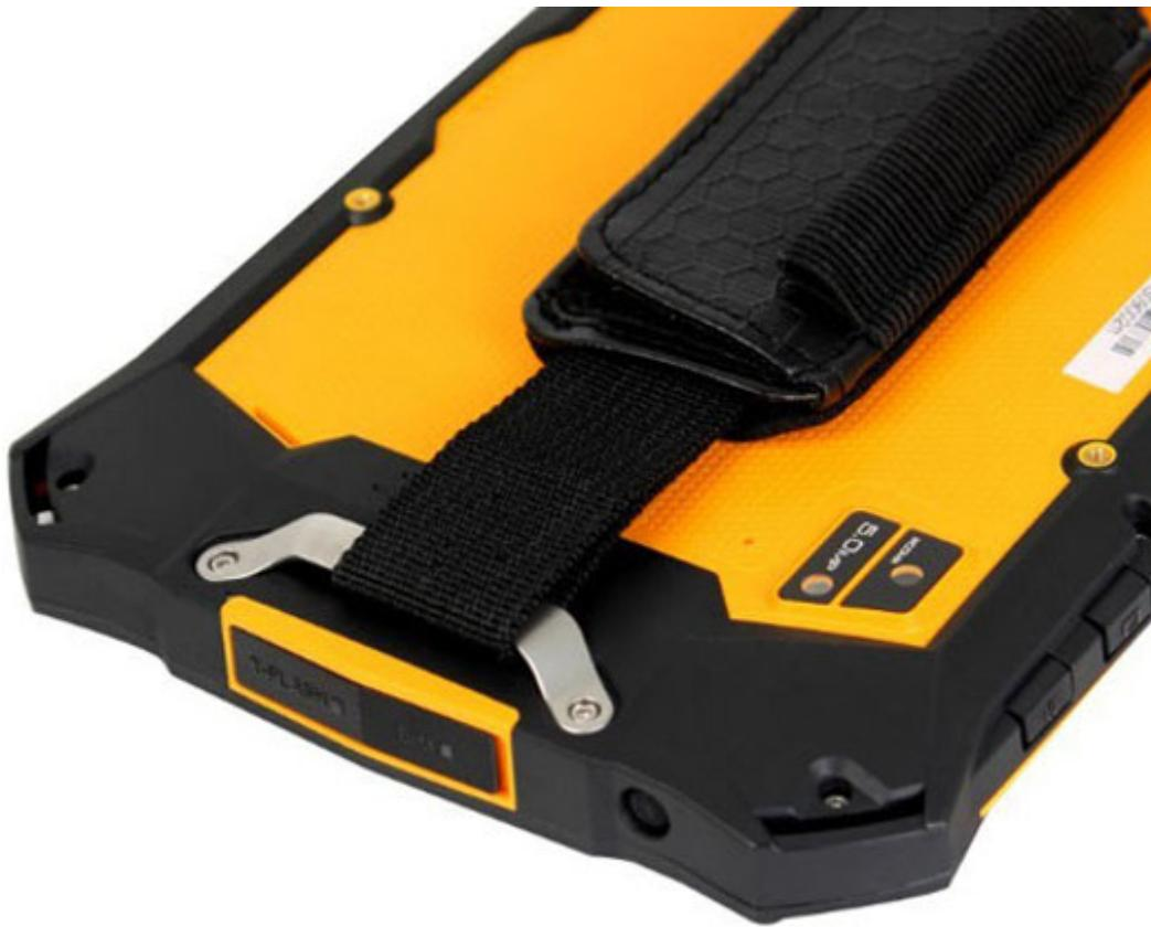
IP stands for Ingress Protection and is essentially a rating system developed by the International Electrotechnical Commission or the IEC. The system is now being used to classify different degrees of protection against intrusion or immersion. The IP rating is usually followed by two digits. The first indicates the level of dust-resistance, the second water resistance. Dust-resistance levels goes from 0 up to 6 while water-resistance goes from 0 to 8.
