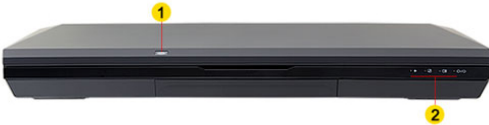
2. Airplane Mode, Touchpad On/Off, Power and Battery Charge Status Indicators
