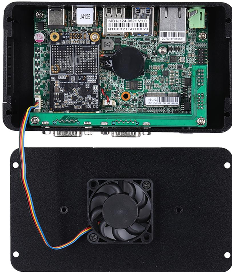
The industrial Mini PC uses a proven cooling system, based on solid elements, mainly heat sinks. However, pc has a small fan which function is redistributing heat evenly across the case, helping heat sinks keep the optimal temperature of the device.
