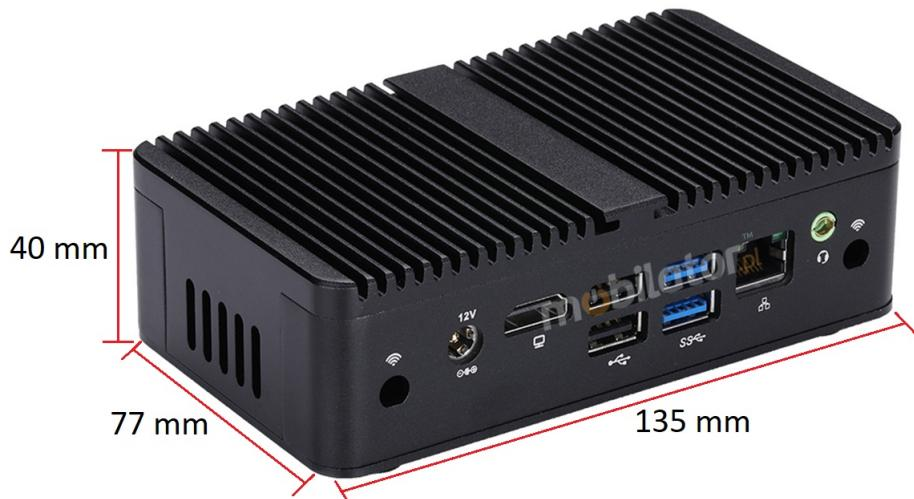
Thanks to the small dimensions of the MiniPC, the is versatile for use at home, in the office and in the industry, for example in the production hall. It's literally everywhere, and thanks to the VESA mount it can be mounted on the back of the monitor to optimize the job.
