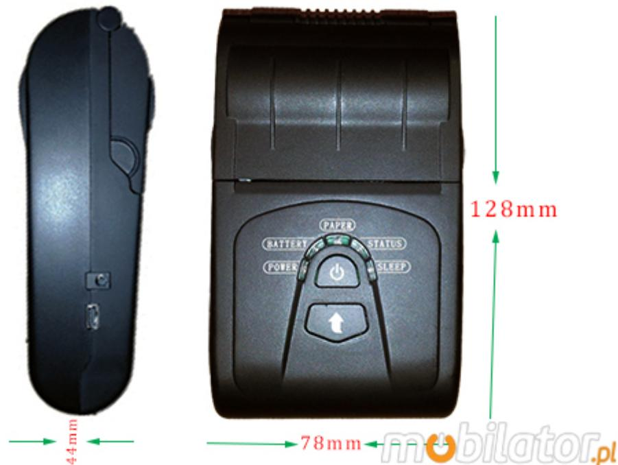
This printer surprises his appearance. This ergonomic, compact and extremely lightweight thermal printer dimensions (128 mm x 78 mm x 44 mm) and weight only 200g, allows complete mobility.
