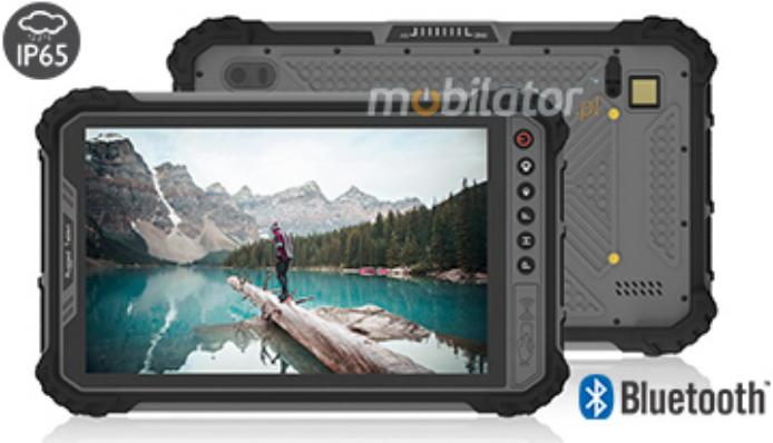
MobiPAD 9TS-M v.9 - a handy and durable industrial tablet with UHF RFID with a range of up to 4 meters, NFC, fingerprint reader, 5Mpx/13Mpx, 8GB RAM and 256GB ROM
