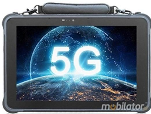
MobiPAD A311-T v.1 - multi-tasking industrial tablet with 8-core processor, Bluetooth 5.0, NFC, Wifi, Android 10.0, 8GB RAM and 256GB ROM
