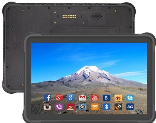
MobiPad Cool A311L v.3 - Industrial, splash-proof (IP65) tablet with UHF RFID and NFC, Bluetooth 4.0, 4G
