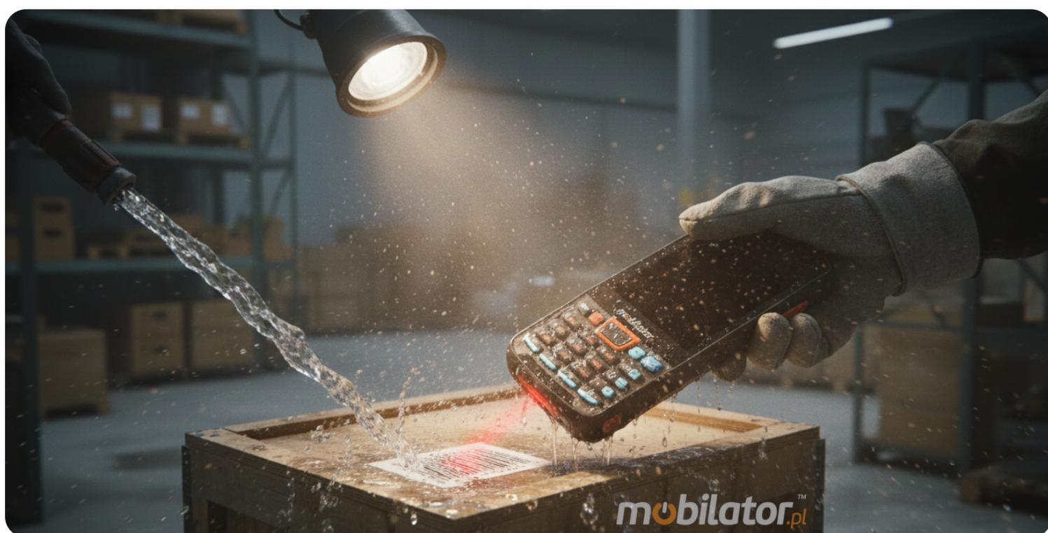
Demanding industrial and field environments require uncompromising protection – and that's precisely what the IP65 standard provides. Meeting this rigorous standard, the special-purpose collector features a completely dust-tight enclosure (number 6) and a high degree of protection against pressurized water jets from any direction (number 5). This ensures the device is protected against
