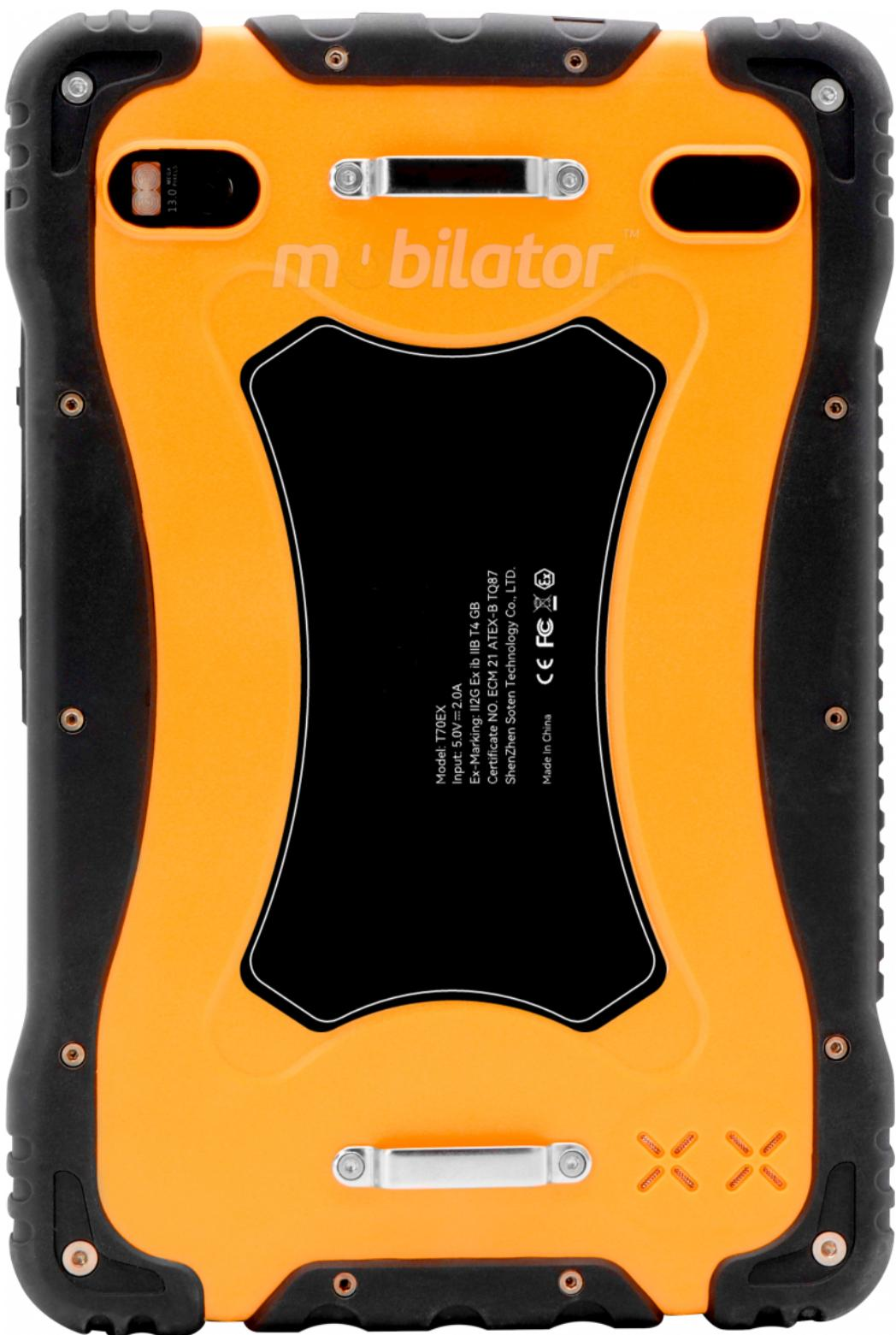
NFC in industrial tablets is a short-range wireless communication technology that enables rapid data exchange between the tablet and another device (e.g., an RFID tag) by bringing them close to each other.
