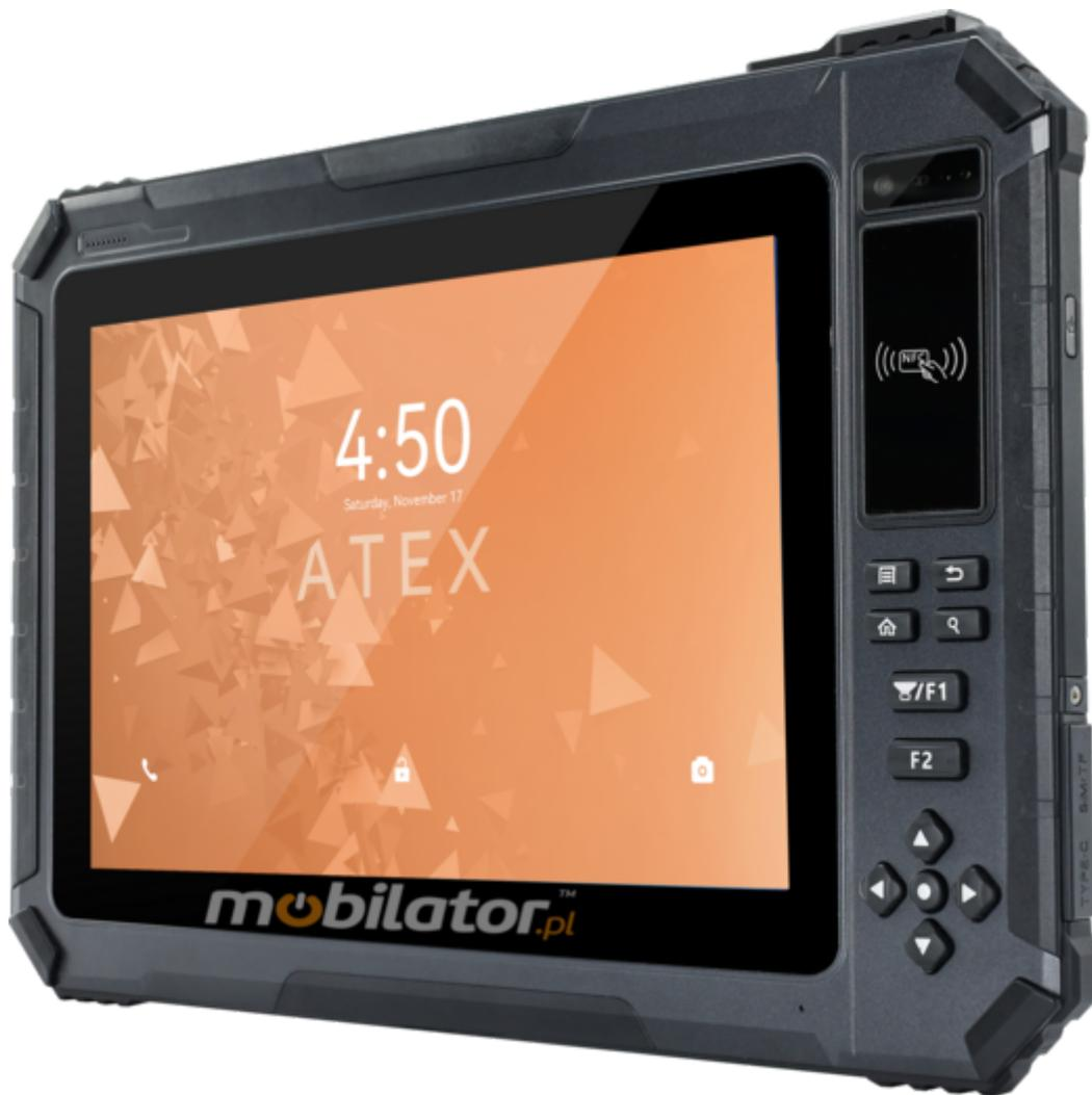
Nit is a unit of measurement used to describe the brightness of electronic device screens – the higher the number of nits, the brighter the display. The MobiPad Tex101 boasts a screen with an impressive maximum brightness of 1000 nits. This level allows for trouble-free use of this dust- and water-resistant tablet, even in direct sunlight.
