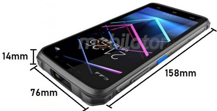
Industrial Data Collector MobiPad TF20-H is designed for resistance and convenience. The sleek and rugged 14mm thick design and stylish case will make the collector very well suited for industrial use and more. The unique size has been carefully thought out to make the device more comfortable and ergonomic. The non-slip casing makes it safe and secure to hold it in your hand.
