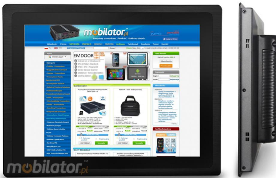
PC Panel is widely used primarily in the commercial industry, for example for controlling the sales system, displaying product information on monitors or advertising on large screens. With the VESA holder in the housing there are many possibilities for its assembly, eg in stores (at the cash register) in factory halls, in a car delivering products, etc. It will certainly be used in all types of retail chains.
