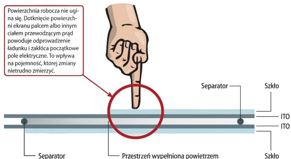
In a capacitive screen, the reaction of the device is not to directly press the surface of the screen, but to change the electrostatic field in the place where the device has been touched. This allows for a much more precise operation and gentle strokes on the screen. In addition, we can use multitouch technology, i.e. the ability to control our totem with several fingers at the same time.
