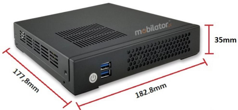
Thanks to the small dimensions of the MiniPC, the is versatile for use at home, in the office and in the industry, for example in the production hall. It's literally everywhere, and thanks to the VESA mount it can be mounted on the back of the monitor to optimize the job.
