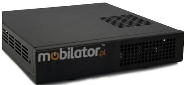
Polywell-HM170L4 i3 v.1 - Industrial miniPC computer in a durable metal housing - with four LAN ports, i3 processor, HDMI, DP and VGA
