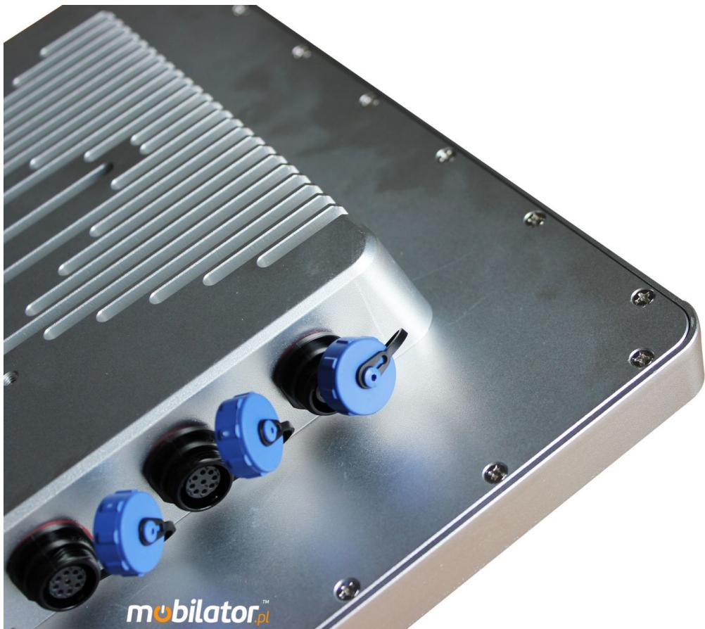
IP norm (International Protection Rating) determines the degree of protection provided by the housing of an electrical device against such factors as: access to dangerous parts inside the housing, penetration of foreign solids and
