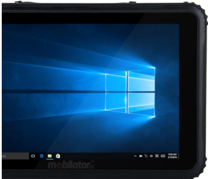
Rugged 8-inch tablet (IP67 + MIL-STD-810G) with NFC, powerful Intel processor, 4GB RAM, 64GB ROM, Bluetooth 4.2 - Emdoor I88H v.2
