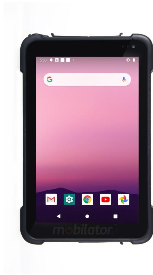
A nit is a unit of measure that describes the screen brightness of all kinds of electronic devices with a display. The higher the number of nits, the brighter the display is. As standard, there is a screen with a maximum brightness of 450 nits. Optionally, you can equip the device with a screen with a brightness of up to 800 nits, which will allow you to work in difficult conditions.
