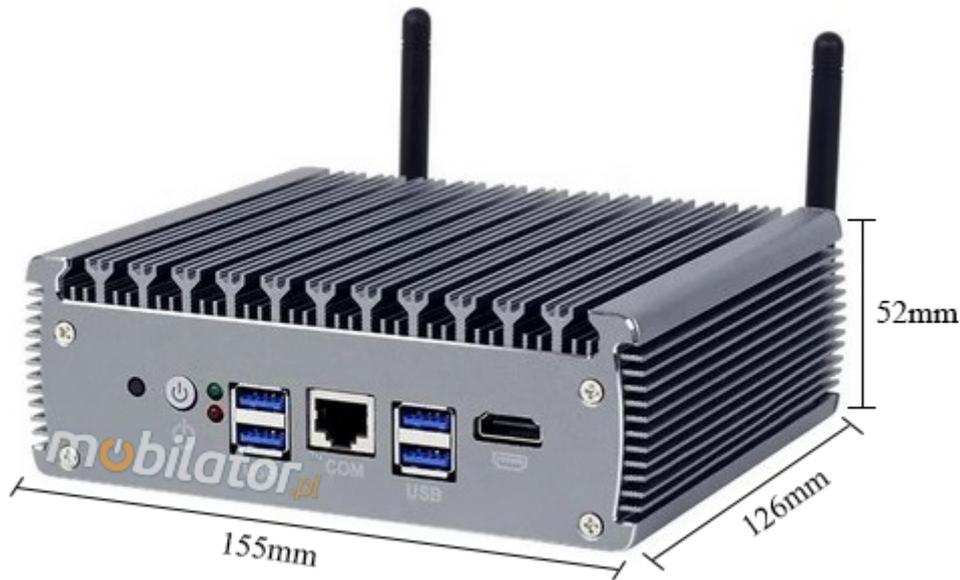
Thanks to the small dimensions of the MiniPC, it is versatile for use at home, in the office and in the industry, for example in the production hall. It's literally everywhere, and thanks to the VESA mount it can be mounted on the back of the monitor to optimize the job.
